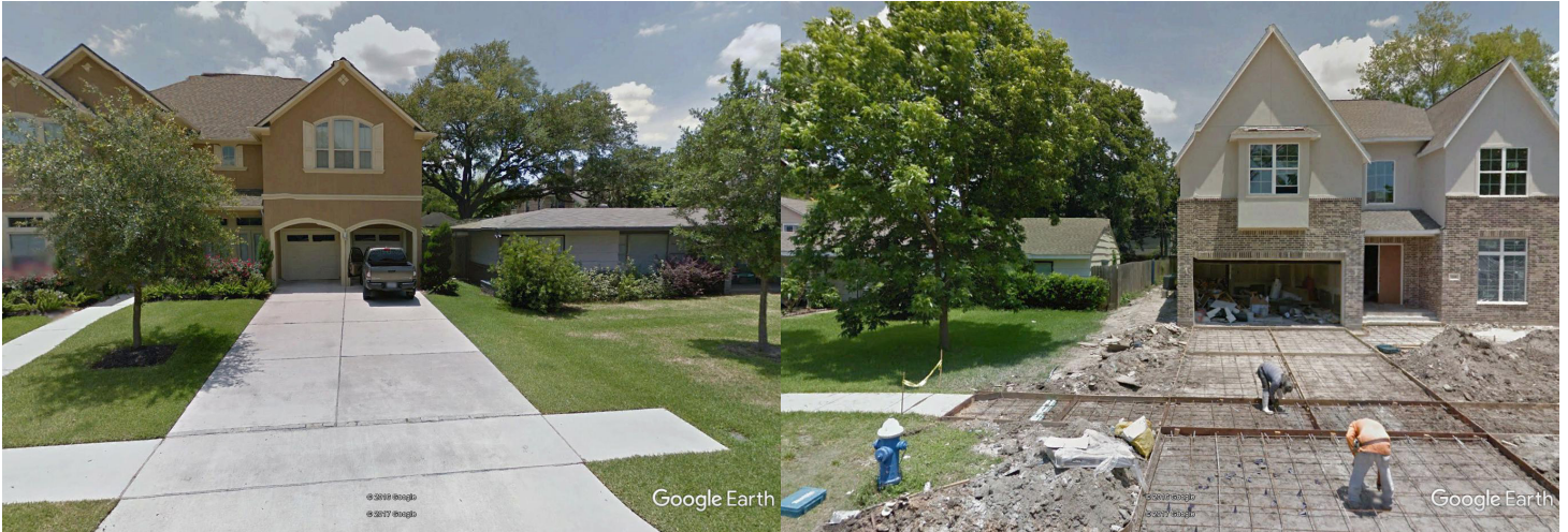
FIGURE 20. LARGE HOMES REPLACE SMALLER HOMES, INCREASING RUNOFF FROM ROOFS AND DRIVEWAYS (HOUSTON). SOURCE: GOOGLE EARTH.
